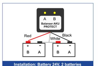
Battery equalizer can be used for 24V, 36V, 48V and any other N\*12V battery system
